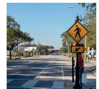
Warns drivers that a pedestrian is crossing at an unsignalized location when flashing signal is activated by the pedestrian.
